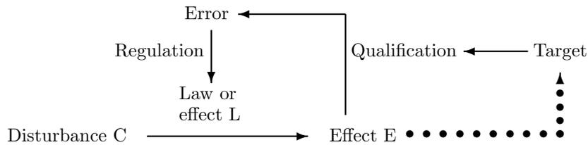
This is the error-controlled regulation diagram which, like the diagram above, specifies cause-effect relations. In addition, a dotted line now indicates that the effect E determines the target of regulation, thereby achieving a “closure”. What Rosen showed, was that the “effect” can not just determine the target, but can be the target, even though this means there is then an impredicative! What does this mean?
